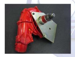
2). Unbolt the Supercharger halves and remove the turbine impeller, **NOTE: This has a left handed thread.** Remove the oring behind it and the step collar. Tap shaft out of the Supercharger housing.
