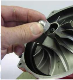
13). Use black high temp sealant to re seal the housing halves and blue thread lock on the bolts holding the housing together. Torque to: **89 inch-pounds not ft pounds.**
