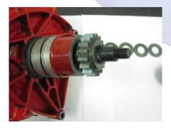
17). Slide the other steel washer (16) up over the shaft, then install the locking washer (17) with the two flat spots for the wrench to hold.
