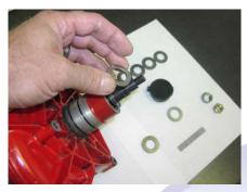
15).Install the larger steel washer (14) first then apply a thin later of the provided grease (22) to the shaft. This will act as an adhesive to hold the needle bearings (15) to the shaft as you install all 40 of them (count them 40).
