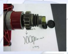
20). Install the L-ring (19) and hex nut (20) (use blue locking agent). Torque nut to **22ft-lbs.**-make sure to hold the locking washer with the retaining wrench provided in the Supercharger tool kit.
