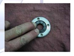
6). Install one of the new bearings into the supercharger housing using the bearing install tool, then screw the retaining disk (9) back into the hosing. Torque this part to 22 ft-lbs.
