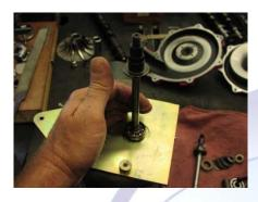
(8). Tap the shaft lightly with a block of wood and a mallet to seat the bearing down and into position.
