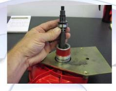
11). Install the step collar (7) and o-ring (5) to the inside section of the Supercharger. (photo below)
