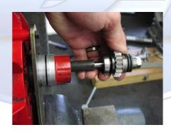
3). Use the 4 pin spanner socket to remove the retaining disk and push the bearing that is located behind the disk out of the housing. It pushes out towards the disk you removed.
